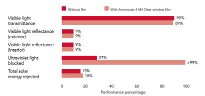
All performance results are based on the film installed on the inside surface of 4mm and 4mm+4mm thick, clear glass
